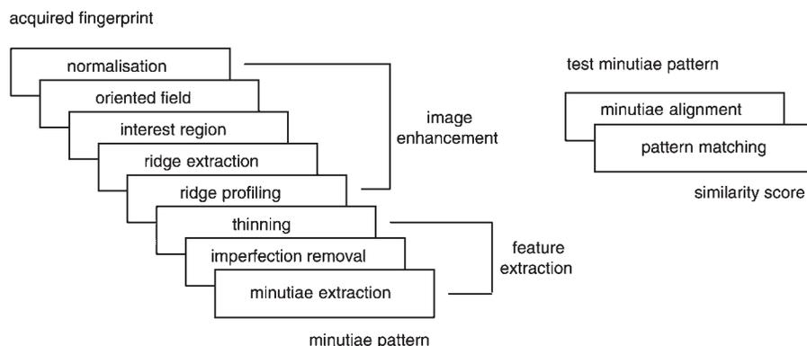
**Fig. 2** Block diagram architecture of the automatic fingerprint recognition system
