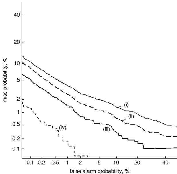
**Fig. 8** DET curves when image quality and position control are considered
