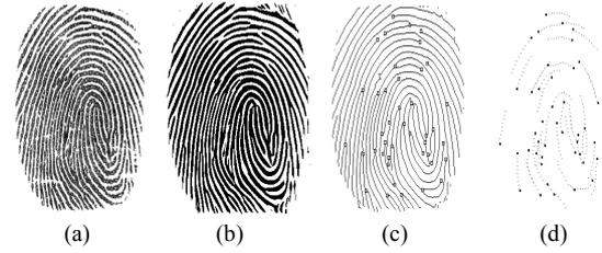
Fig. 2. (a) “*dp\_0080\_0\_5*” MCYT fingerprint. (b) Binary image after image enhancement. (c) Reconstructed thinned ridge structure and extracted minutiae. (d) Extracted minutiae and sampled ridge segments which constitute the biometric pattern of the fingerprint.
