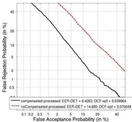
Fig. 5: Pooled DETs (EERs in %) with acoustic dot-scoring system with and without FA channel compensation on ATVS-Dev09 prior to  $t$ -normalization. 30s test segments.
